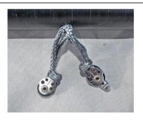
Fold vang strop, leaving one half 200mm longer than the other.
